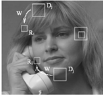
Fig. 1: The transform between domain block ( D_i ) and range block ( R_i )
