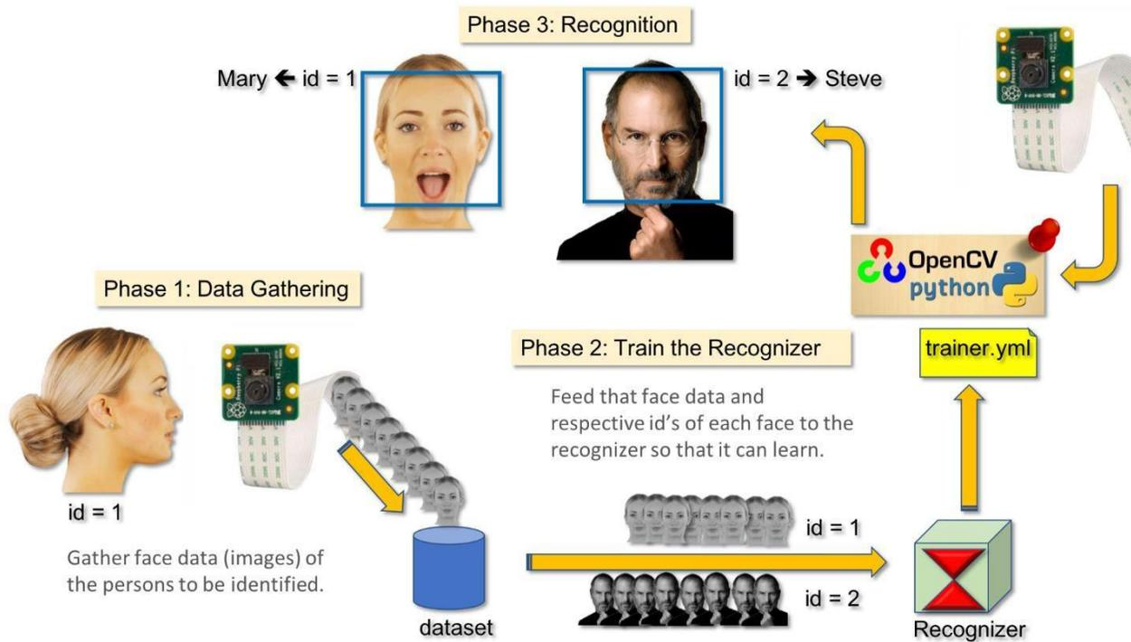
Figure 4.1: Face Detection and Recognition Steps.
