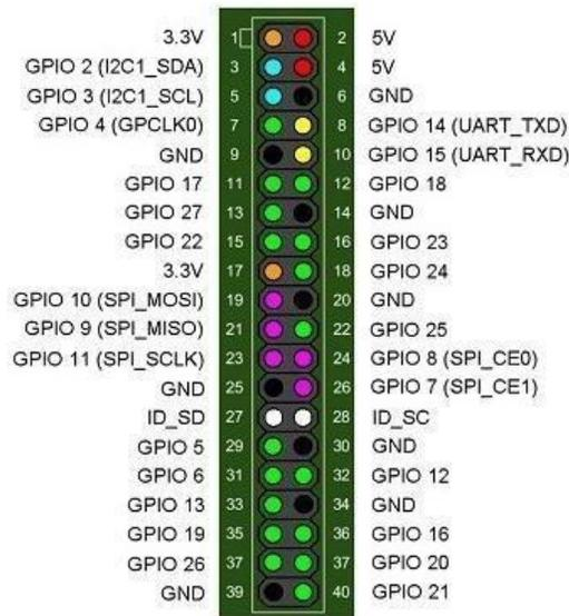
Figure 3.5: Raspberry Pi B+ pins.
