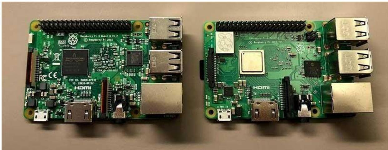
Figure 3.4: Raspberry P 3 B and Raspberry P 3 B+.
