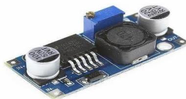
**Figure 3.9:** LM2596 voltage regulator.
