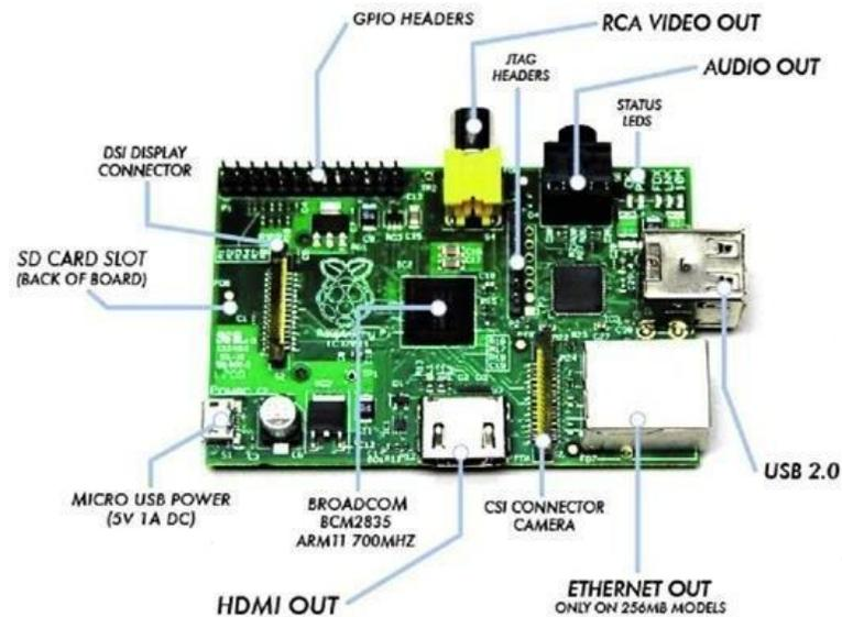
Figure 3.3: Raspberry Pi with important details.
