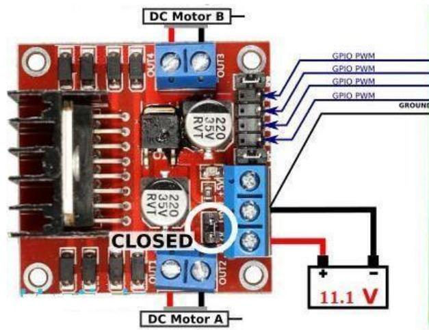
**Figure 3.10:** DC motor Driver connections.
