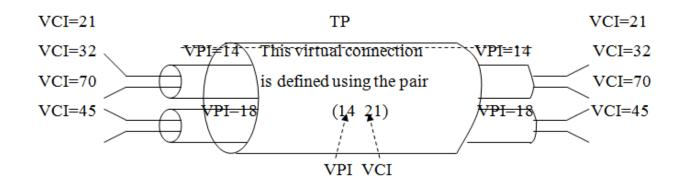
The lengths of the VPIs for UNI and NNI are different. In a UNI interface, the VPI is 8 bits, whereas in an NNI is 12 bits. The length of the VCI is the same in both interfaces (16 bits). We therefore can say that a virtual connection is identified by 24 bits in a UNI interface and by 28 bits in an NNI interface.
